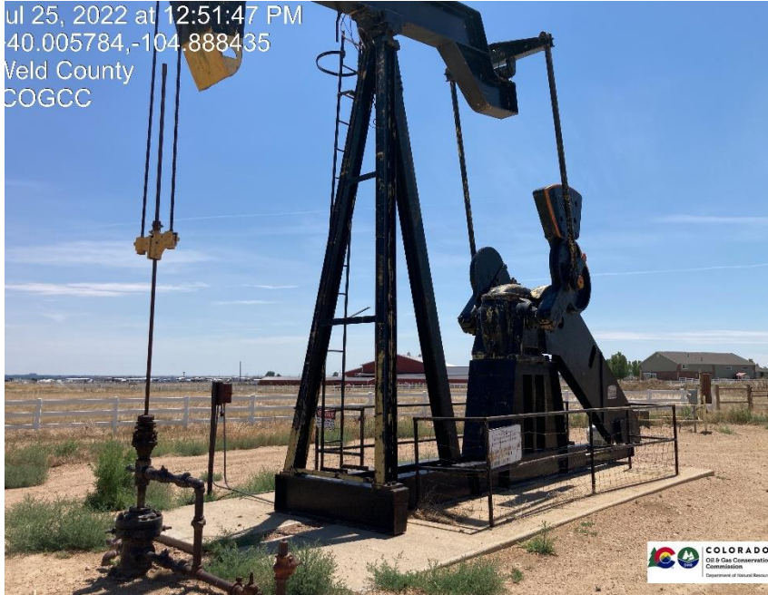
Pic 1 wellhead / pump jack
