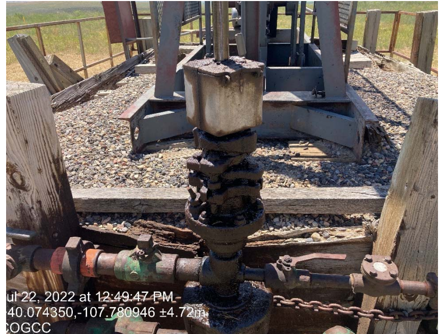
Leaking stuffing box
