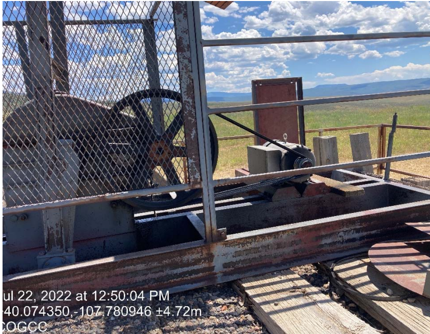
Belt on pump jack lacking cover
