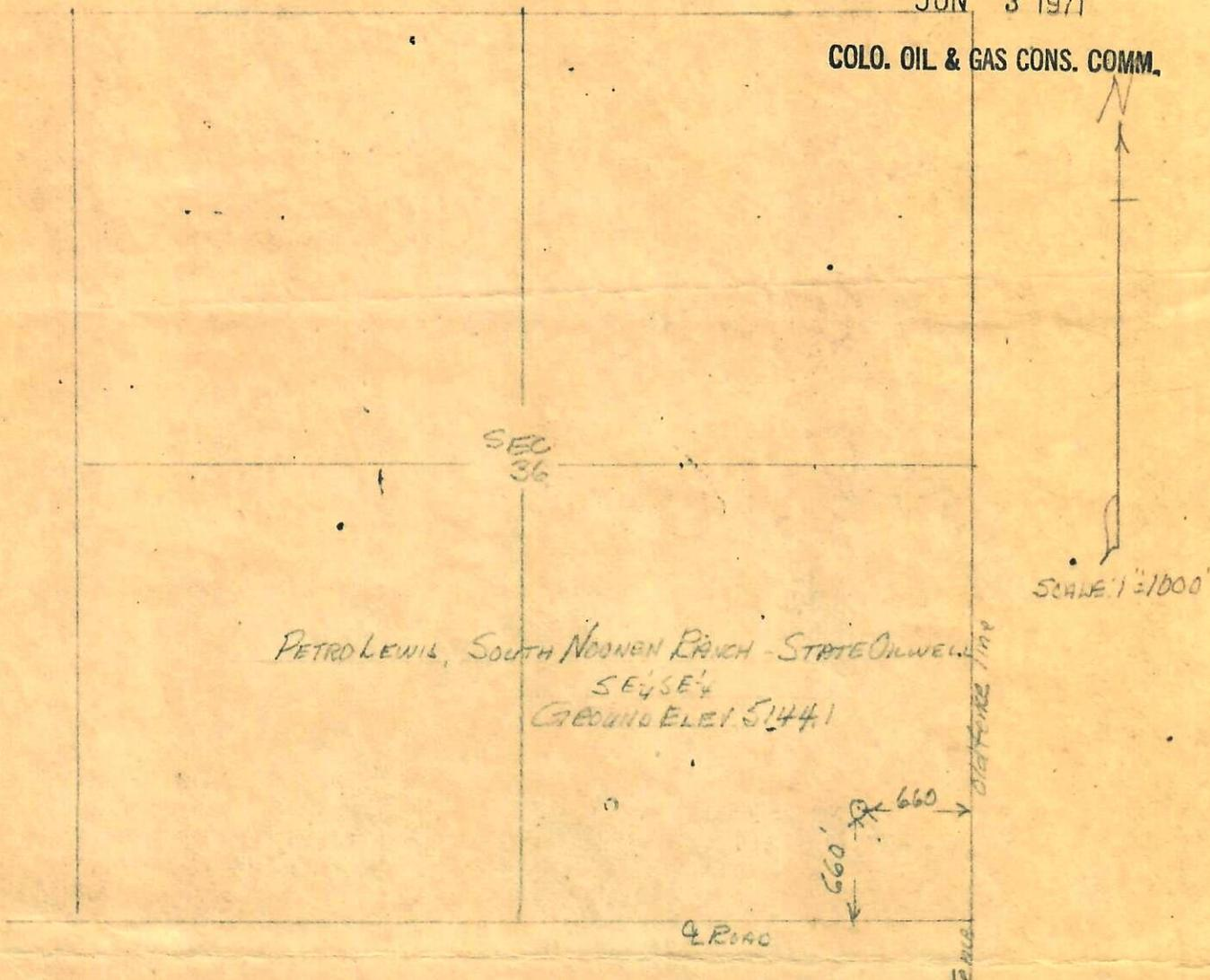
I hereby certify that the above plat is an accurate representation of a correct survey showing the location of Petro Lewis South Noonan Ranch STATE No. 16-36 Oilwell in SE  $\frac{1}{4}$  SE  $\frac{1}{4}$  Sec. 36 T3S R59W 6PM. The elevation of the ground at the stake is 5144.1 feet above sea level from U.S.C.&G. Bench Mark.
