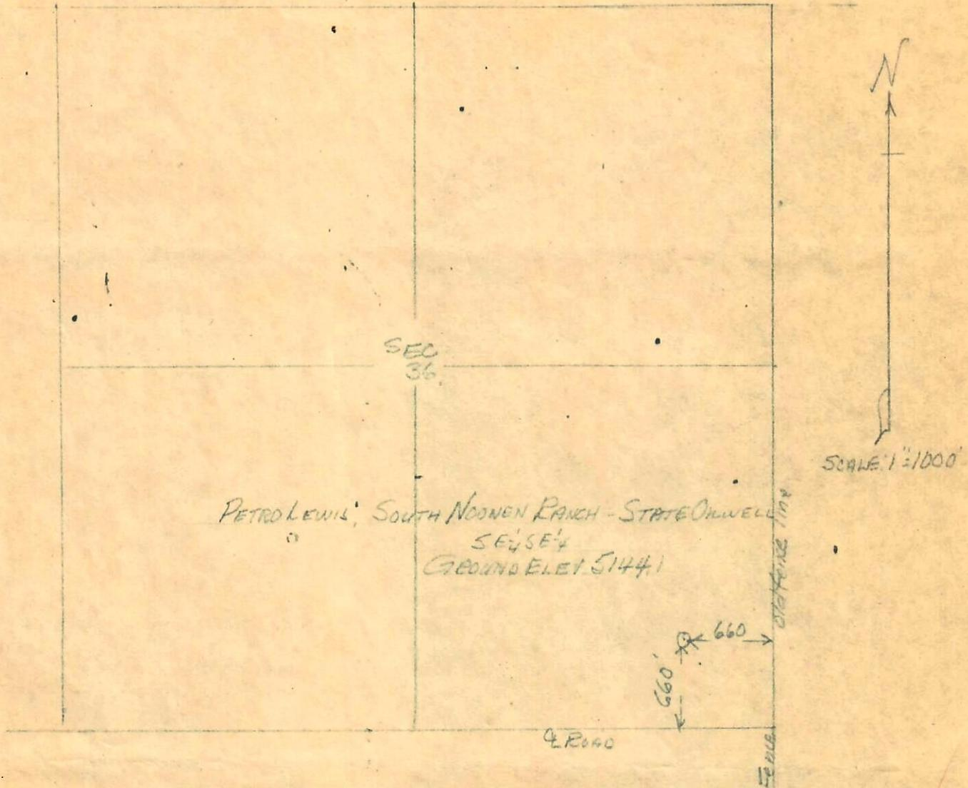
I hereby certify that the above plat is an accurate representation of a correct survey showing the location of Petro Lewis South Noonen Ranch STATE N 1/4-3/4 Oilwell in SE 1/4 SE 1/4 Sec. 36 T3S R59W 6PM. The elevation of the ground at the stake is 5144.1 feet above sea level from U.S.C.&G. Bench Mark.
