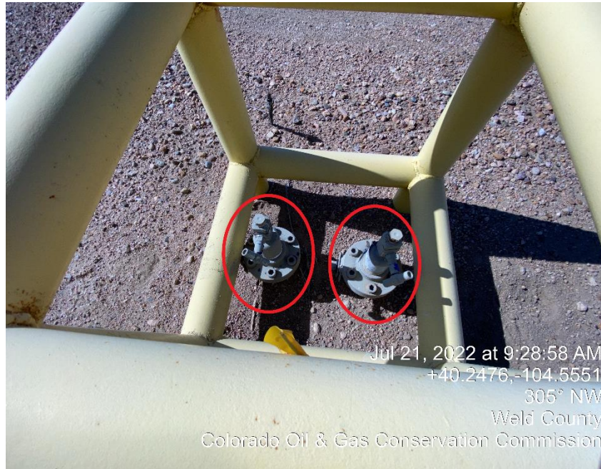
Photo #2 Unmarked Riser
