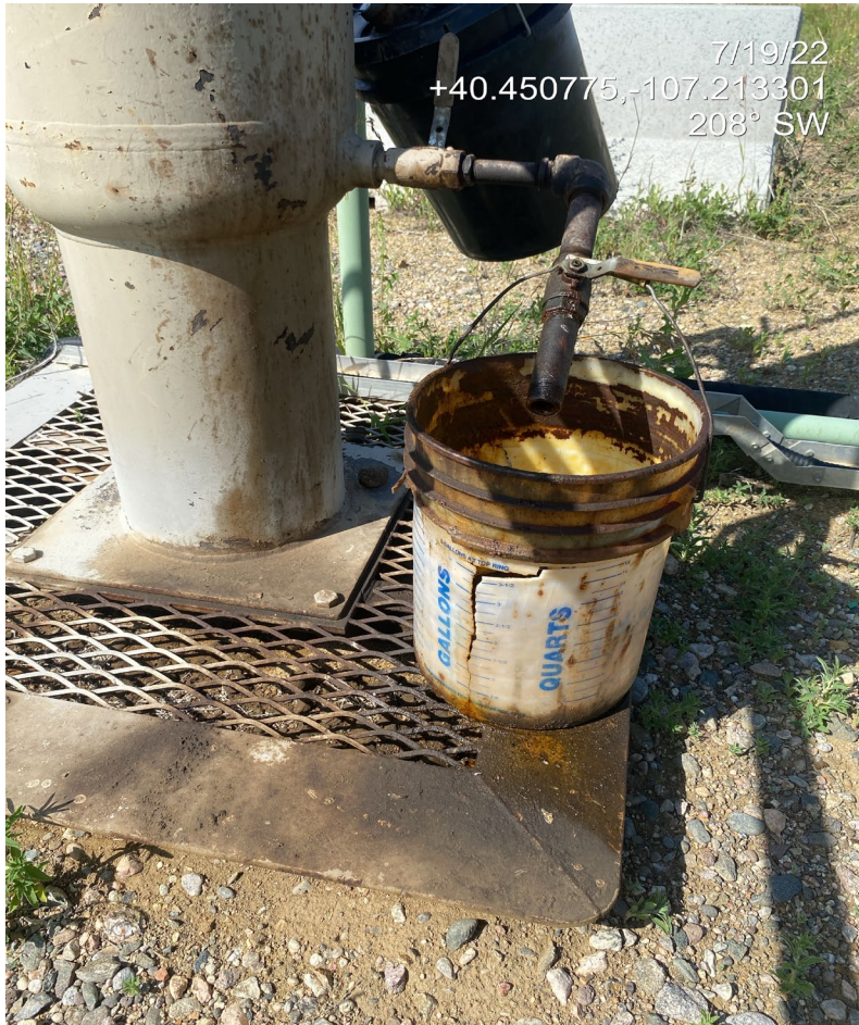
Photo 10. Photo taken from the north of the Location shows fluid dripping from production equipment into an inadequate container. Impacted/stained soils were present beneath the container.
