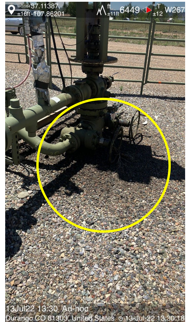
IMG 04 Lube oil has impacted surface material
