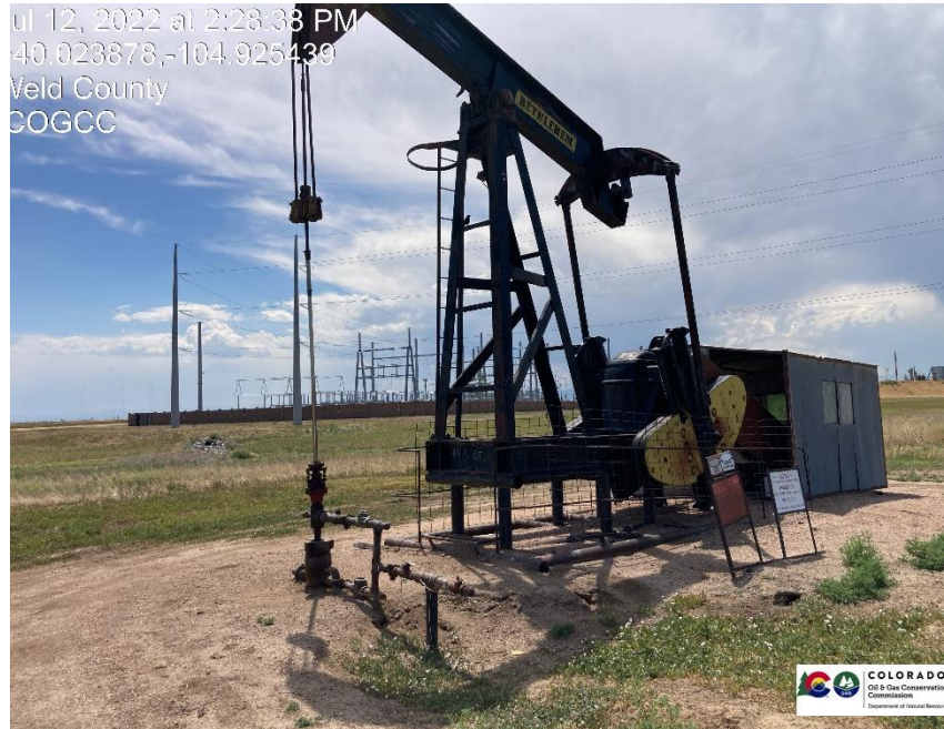
Pic 1 wellhead / pump jack
