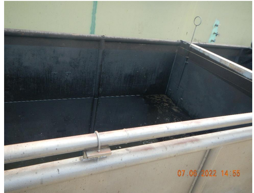
Crude oil in open top tank. No netting for wildlife protection.
