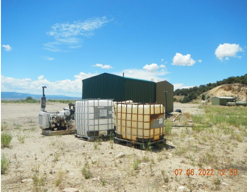
Unused supplies and equipment stored on location. Chemical totes with no secondary containment.
