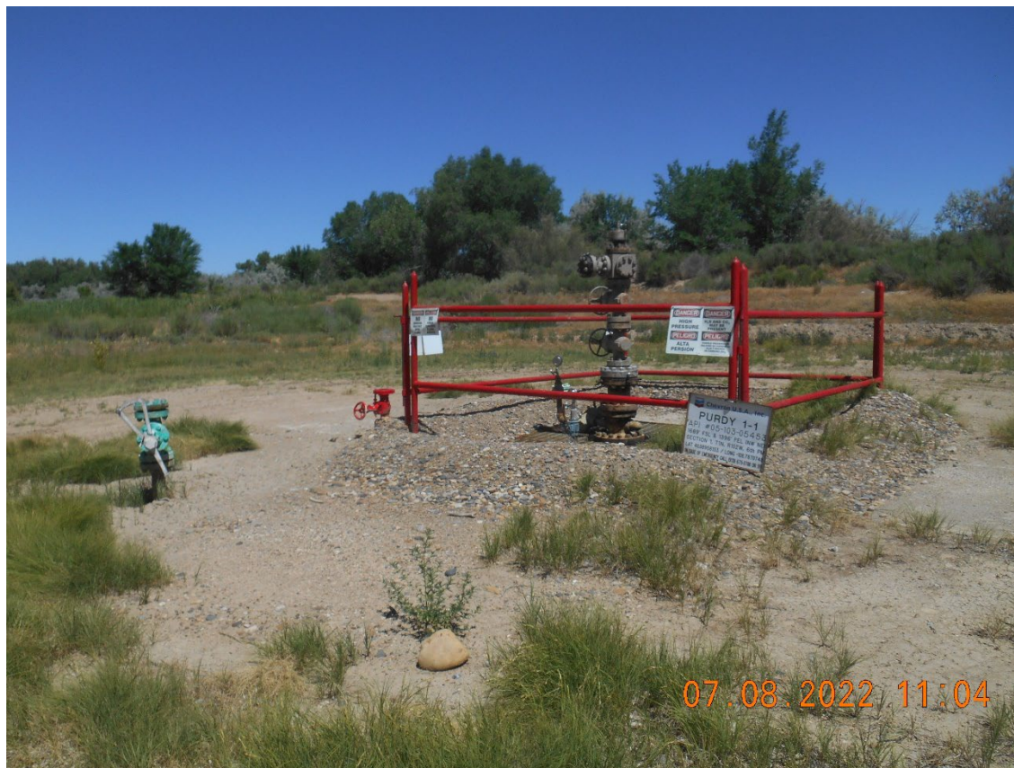
Injection wellhead. Temporarily Abandoned.
