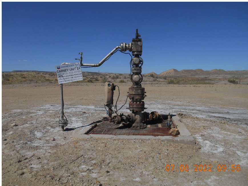
Injection wellhead
