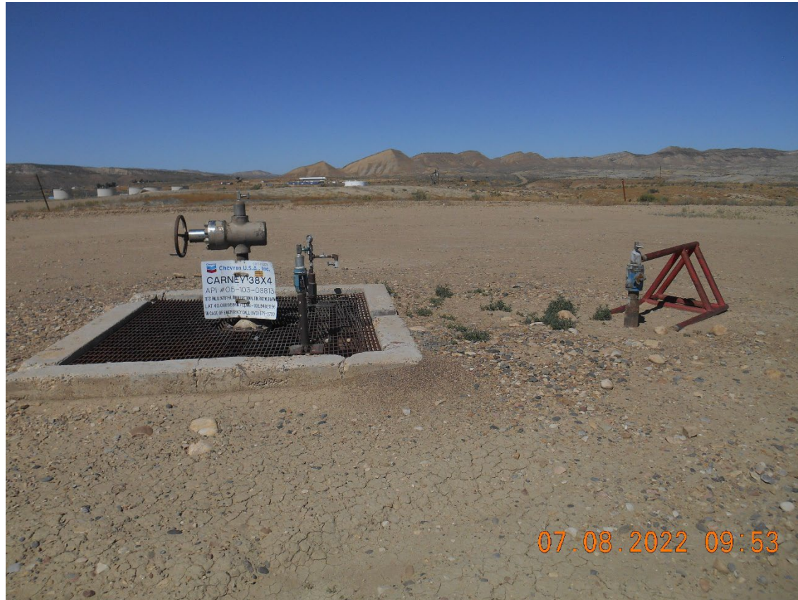
Injection wellhead. Temporarily Abandoned
