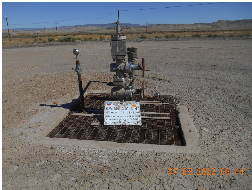
Injection wellhead
