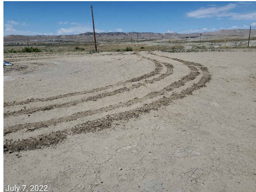
Photo 3: Photo shows vehicle tracking/rutting evident on the pad. Control measures to minimize degradation and sediment transport are missing or insufficient at the Location, and the two access roads leading south and west from the Location
