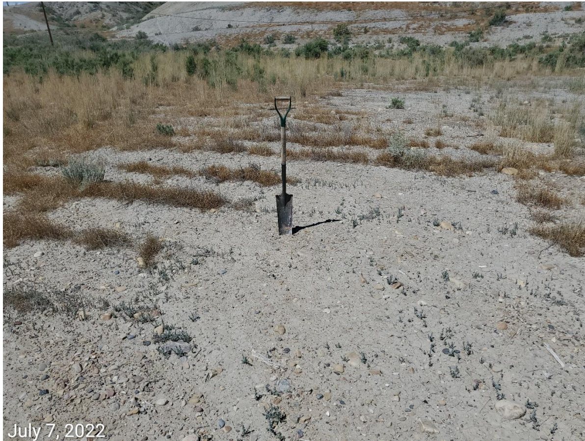
Photo 4: Photo taken from the bare areas of the Location. Photo shows Reclamation Specialist attempted to dig a test pit, but was only able to easily penetrate the first couple inches of soil. Compaction concerns evident at the Location and access road; compaction alleviation inadequate and does not appear to have been conducted.
