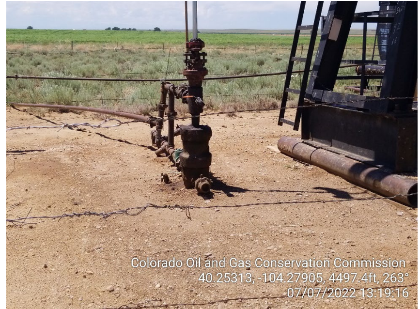
Photo 6 – Stained Soil at Wellhead
