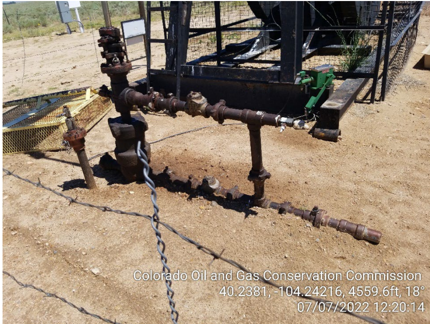
Photo 9 – Stained Soil at Wellhead
