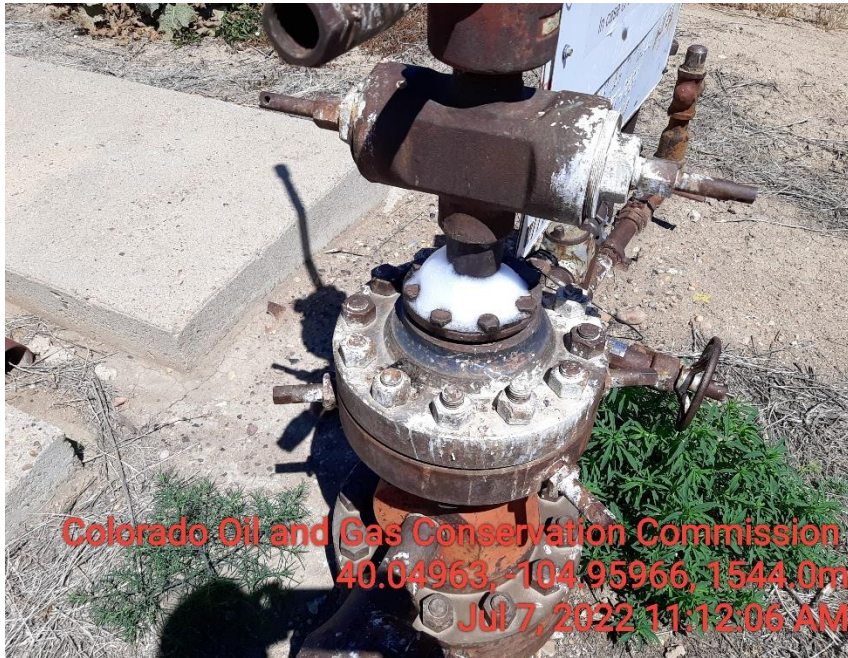
Photo 5 Small leak on well head around tubing.
