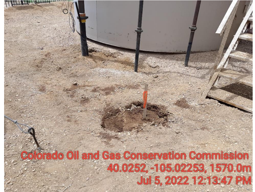
Photo 4 unreported leak or spill between produced water tank and crude oil tank. Stained soil
