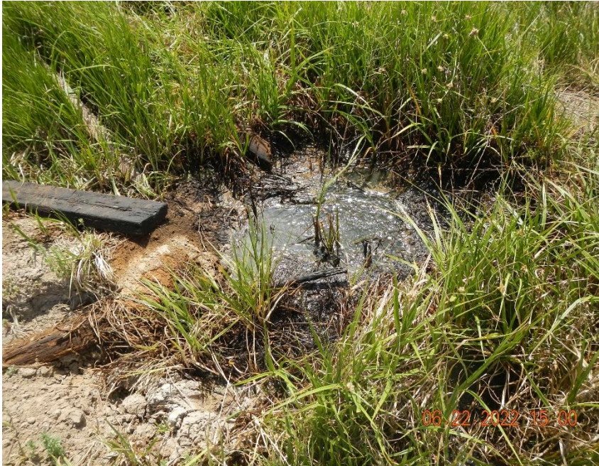
View of fluids and gas bubbles in the vicinity of the Canfield #1.
