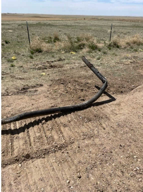
11 – Kummer PC LE 23-99HZ flowline section, 3" carbon steel, good condition, black non-ACM coating
