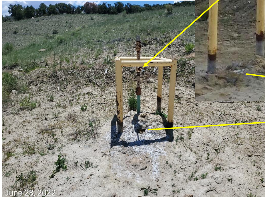
Photo 1: Photo shows riser observed on the west end of the Location, near the entrance. Fluids observed leaking from the riser resulting in a spill and impacts. Salt accumulation evident at point of release- middle photo taken from the 4/22/2021 inspection, and shows that the same accumulations are evident within past inspections, suggesting spill may have been on-going for at least a year
