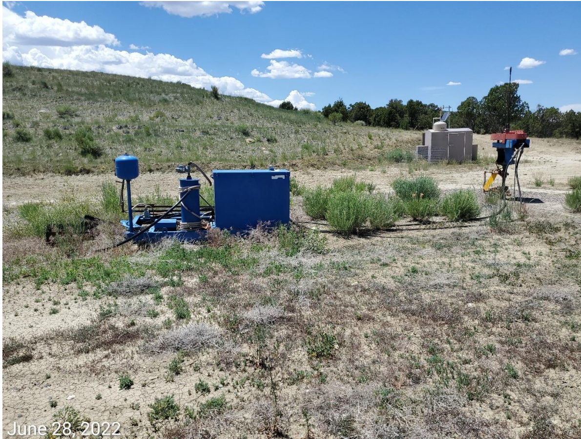
Photo 3: Photo example showing vegetation establishment around production equipment- this is a fire hazard.
