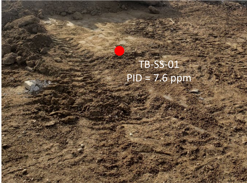
Looking south Former production tank location / connection point No petroleum hydrocarbon staining or odor observed
