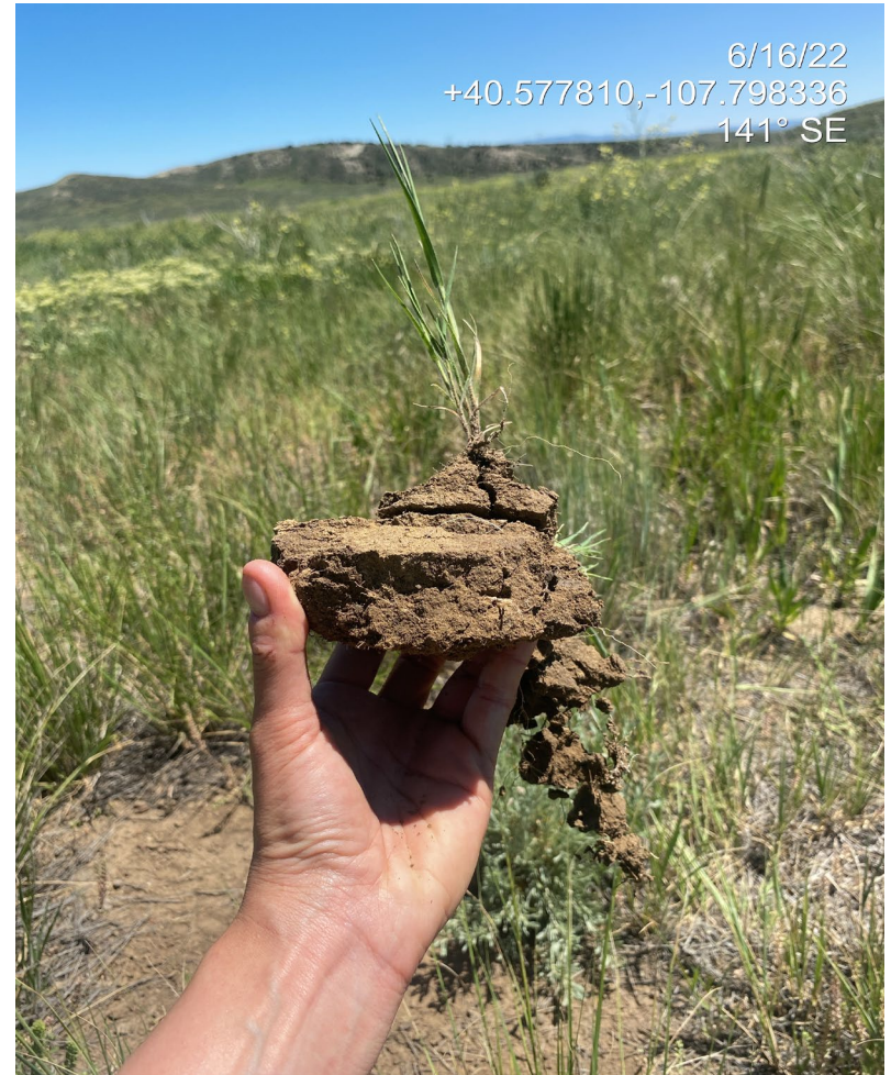
Photo 15. Photo taken from the center of the Location shows a compacted soil layer.
