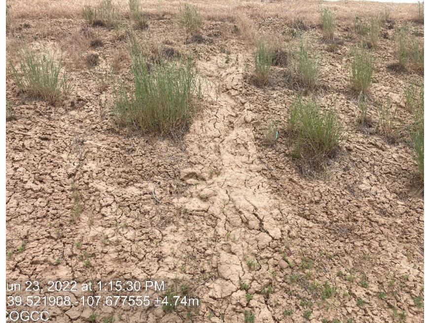
Lack of stabilization/ erosion
