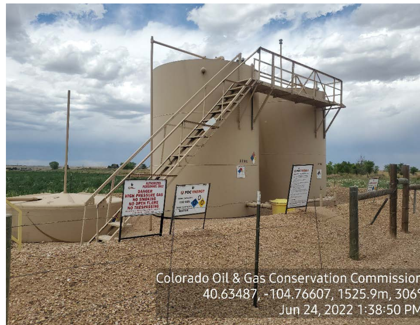
Photo 2: Tank Battery
