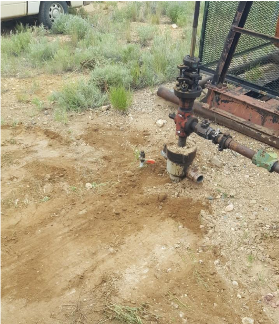
Figure #1 Bradenhead access has been installed.
