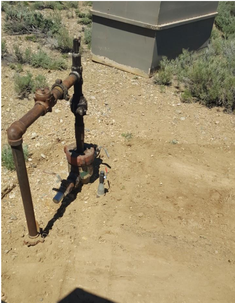
Figure #1 Bradenhead access has been installed.
