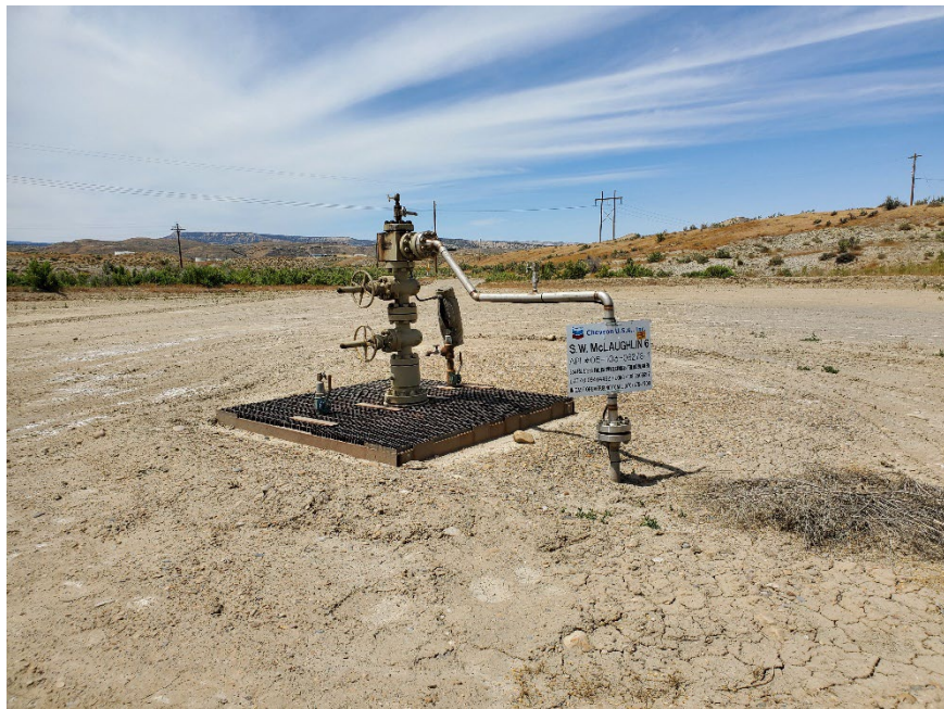
Injection wellhead
