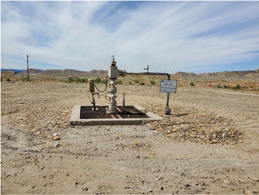
Injection wellhead.
