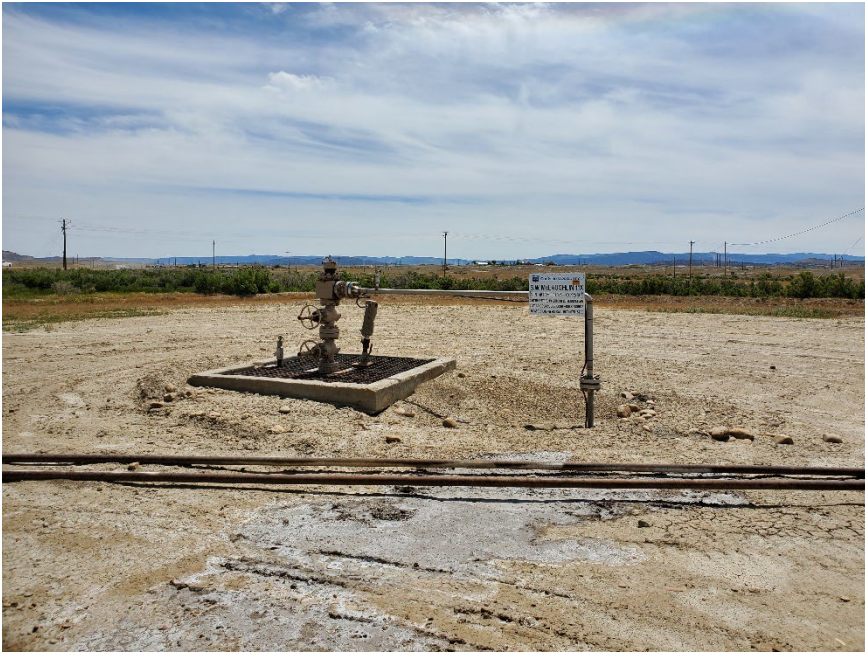
Injection wellhead
