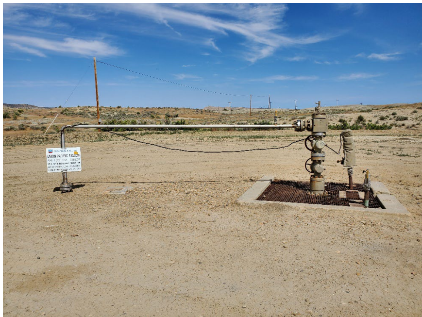
Injection wellhead
