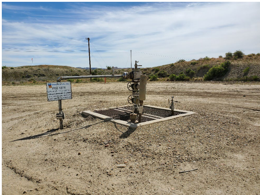
Injection wellhead
