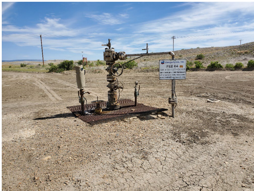
Injection wellhead
