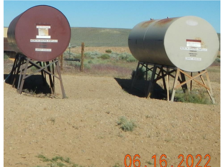
Metal tanks between separators NFPA and capacity are faded.
