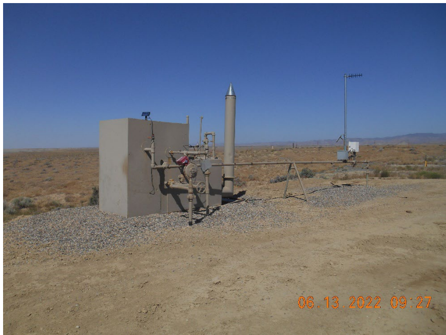
Separator with meter
