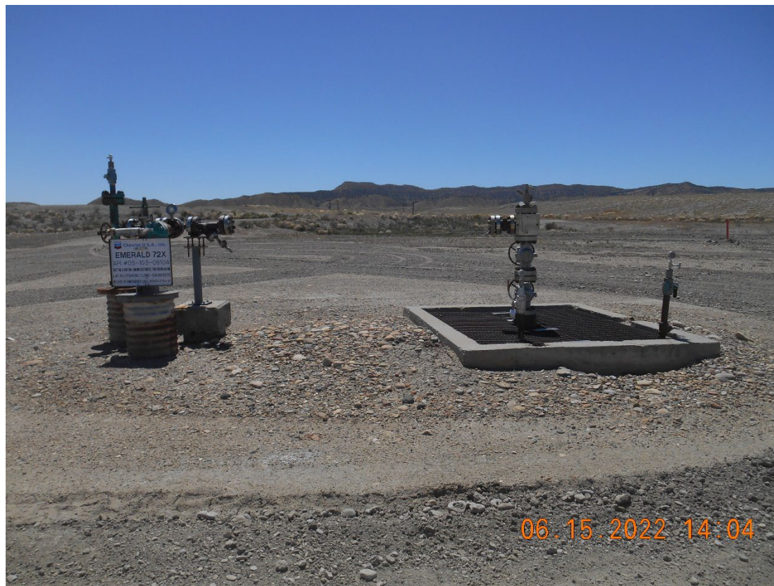
Injection wellhead. Temporarily Abandoned.
