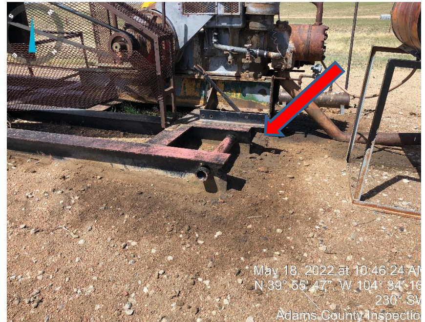
Photo #6 A Stained soil around pump jack.
