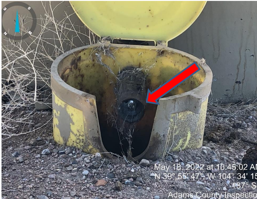
Photo #3 Load off line missing bullplug.
