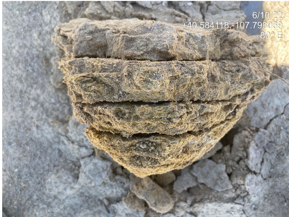
Photo 4. Photo taken at the south of the Location shows platy soil structure indicating compacted soils. Soils were firm compared to adjacent undisturbed areas.
