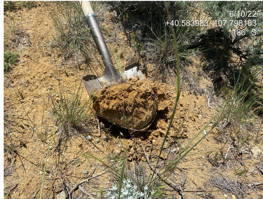
Photo 5. Photo taken to the south of the Location in adjacent undisturbed areas shows loose, granular and subangular blocky soil structures.
