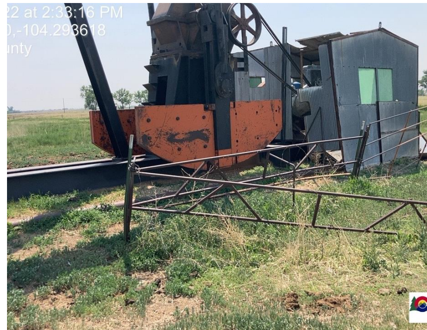
Pic 6 fence around pump jack needs repair
