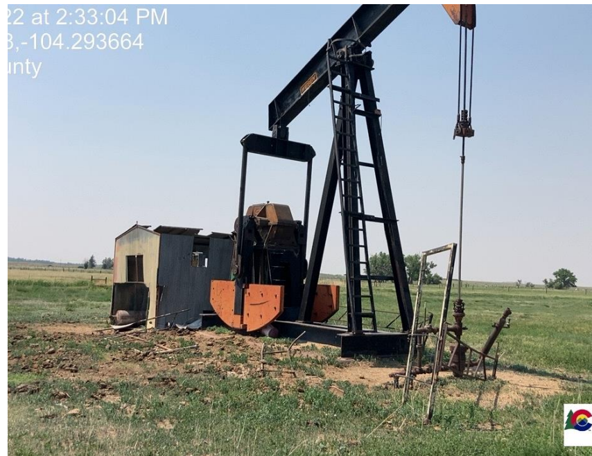
Pic 5 wellhead fence around pumpjack needs repair, motor house needs repair
