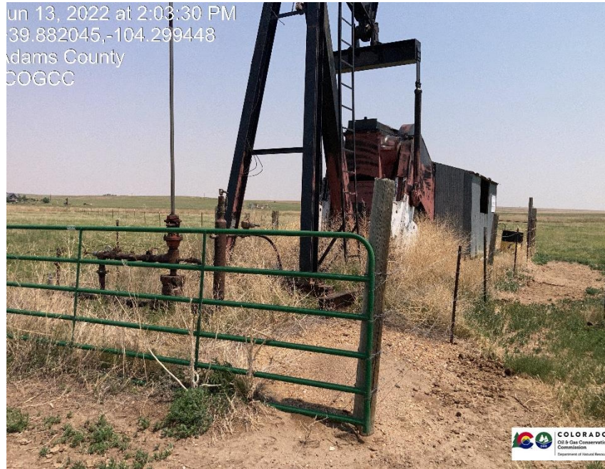
Pic 1 no bradenhead plumbed to surface, stained soil, weeds unmanaged
