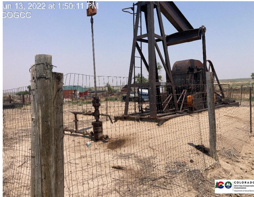
Pic 1 stained soil by wellhead needs to be removed.
