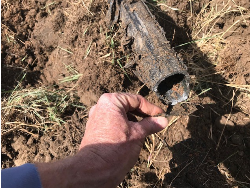
#7 – Steel 2" Diameter Flowline with Tape Coating
