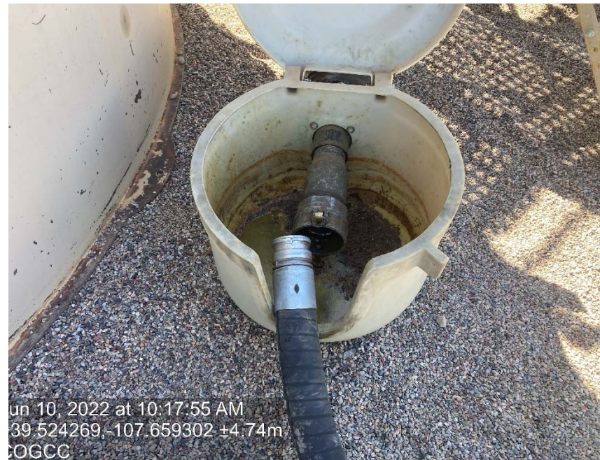
Valve missing cap/ plug
