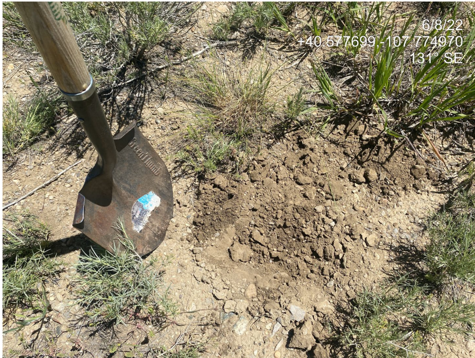
Photo 9. Photo taken from the center of the Location shows highly compacted soils.
