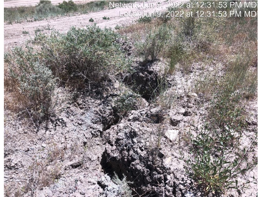
Photo #6876 Gully erosion occurring on cut slope.
