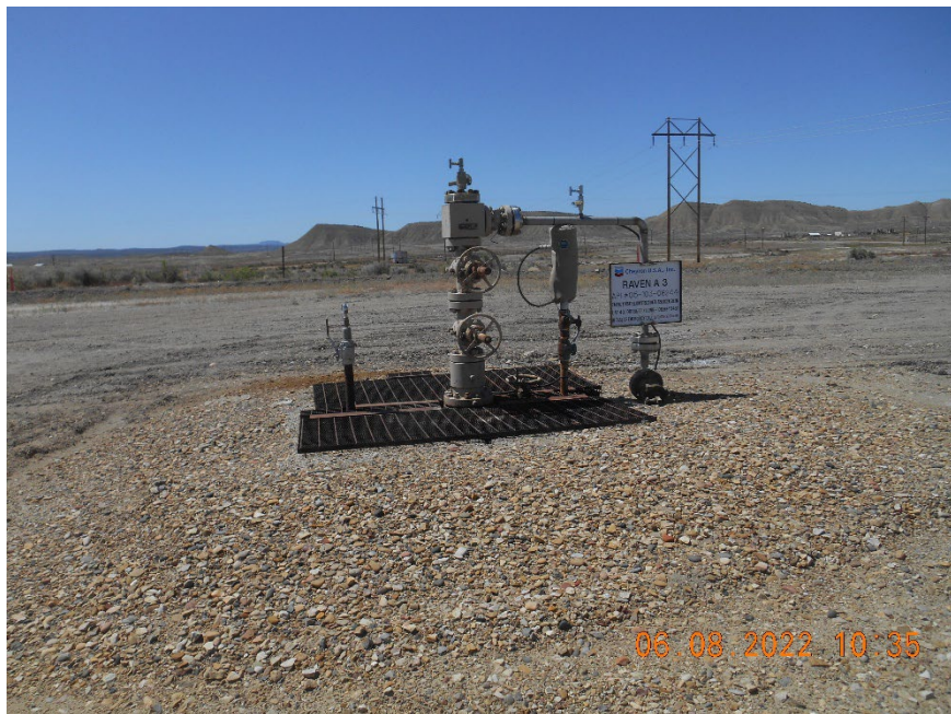
Injection wellhead.
