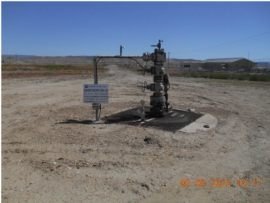
Injection wellhead
