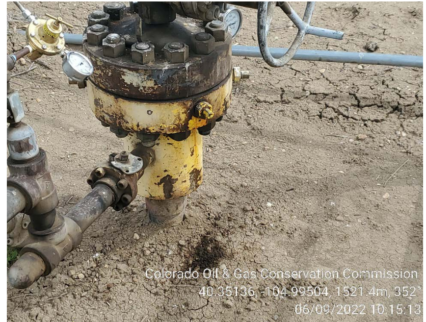
Wellhead leak and stained soil
