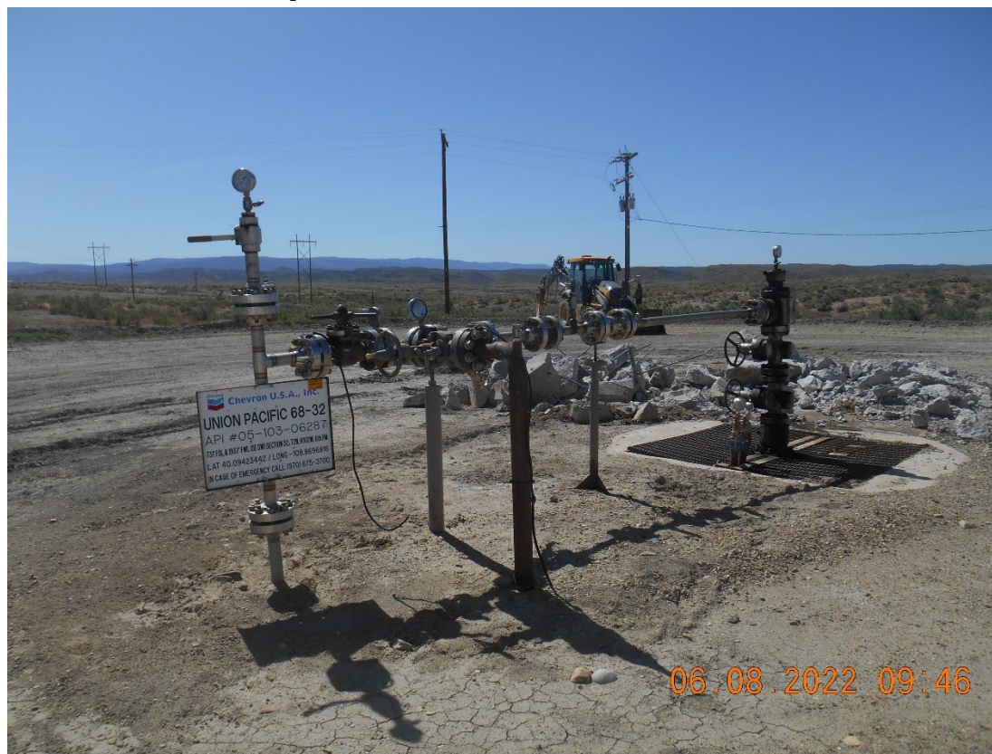
Injection wellhead.
